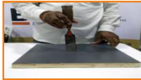
Step 3 : Do not use FARSI to scratch the sheet.
