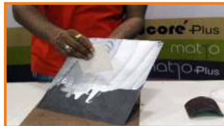
Step 7 : Apply THIN layer of the glue on the surface of the sheet which has been scratch.
